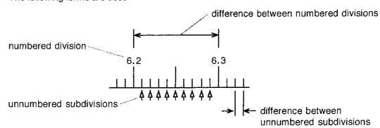
Both the numbered divisions and unnumbered subdivisions are **CALIBRATED** DIVISIONS because the overall scale has been "marked off" or "calibrated" at regular intervals.
